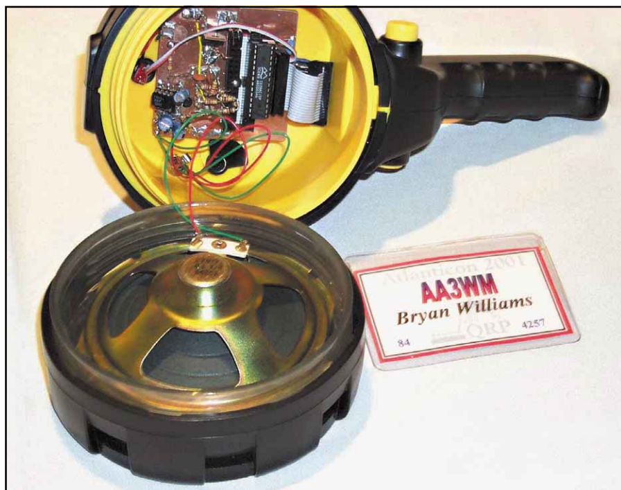
Bryan Williams, AA3WM, built his PSK31 Beacon kit into the shell of a flashlight, providing ultimate portability!
