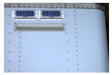
•**TRAILERS, >60,000 in Production** 1 x PVs, Solar Augmented 2 x PVs, 100% Solar w/o Sensors
