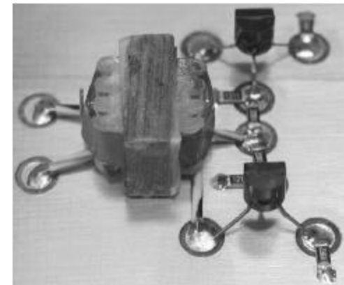
Close-up of the transformer and transistor mountings.
