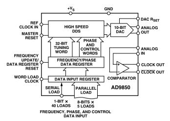
combination thereof. The AD9850 also contains a high speed comparator that can be configured to accept the (externally) filtered output of the DAC to generate a low jitter square wave output. This facilitates the device's use as an agile clock generator function.
