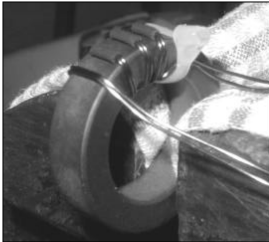
Picture 3: Balun core in vise showing heat shrink tubing on outside of windings.
